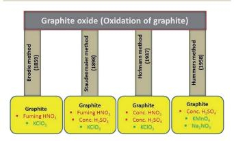
Fig. 1 Methods for synthesis of graphite oxide using graphite, acids and oxidizing chemicals.
