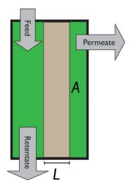
Fig. 8 Schematics of a membrane where feed is the flue gas that enters the membrane with a pressure  $p_{\rm F}$  and composition  $x_{\rm CO_2}^{\rm F}$ . Most membranes have a higher permeability for  $CO_2$  and therefore the permeate is rich in  $CO_2$  ( $x_{CO_2}^p$ ) while the retentate is  $CO_2$  poor (figure adopted from Smit et al.3).
