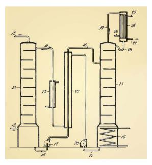
Fig. 6 The original design by Bottoms<sup>7</sup> of an amine scrubbing using the removed  $CO_2$  from natural gas. The current technology for liquid absorption looks very similar: flue gas is injected at (12) and the  $CO_2$  is captured by an amine solution is the absorber (10). In the stripper (15) the amine solution is regenerated using steam (18) from the power plant. Heat losses are minimized by using a heat exchanger (27).
