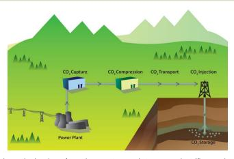
Fig. 1 Schematic drawing of a carbon capture and storage project (figure adopted from Smit et al.<sup>3</sup>).
