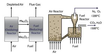
Fig. 5 Chemical looping: the left figure shows the schematics of metal oxide (MeO) used to transport oxygen form the air into the reactor. The right figure illustrates how this solid is looping form the air reactor to the fuel reactor and back (figure adopted from Smit et al.3).
