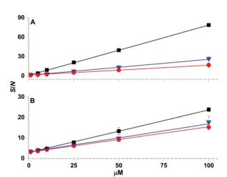
Fig. 5 Solid-phase microextraction low temperature plasma mass spectrometry calibration curves obtained by sampling 1  $\mu$ L of (A) aqueous solutions and (B) synthetic urine containing 1 to 100  $\mu$ M of organophosphates 4 (squares), 5 (triangles) and 6 (circles).
