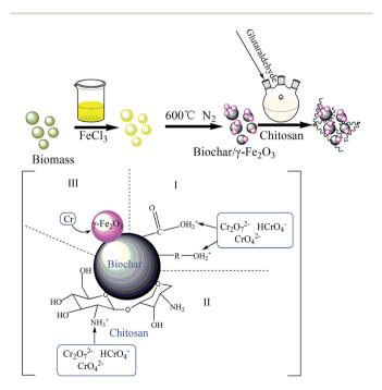
Fig. 1 Schematic representation of strategy for preparation of CMB and  $Cr(v_i)$  removal by CMB.
