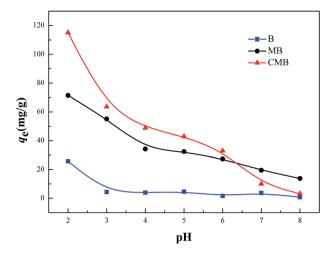
Fig. 8 Effect of the initial solution pH on adsorption of Cr(vi) by B, MB and CMB (reaction conditions:  $c_0 = 150 \text{ mg L}^{-1}$ ; V = 50 mL;  $m = 50 \text{ mg}; t = 6 \text{ h}; T = 30 ^{\circ}\text{C}$
