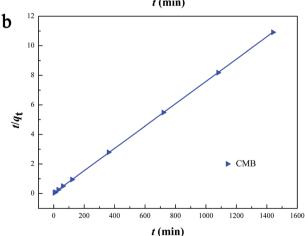
Fig. 10 (a) Effect of contact time of Cr(vi) adsorption onto CMB and (b) pseudo-second-order sorption kinetics of Cr(vi) adsorption onto CMB (reaction conditions:  $c_0 = 200 \text{ mg L}^{-1}$ ; V = 50 mL; m = 50 mg; pH = 2;  $T = 30 \, ^{\circ}\text{C}$ ).
