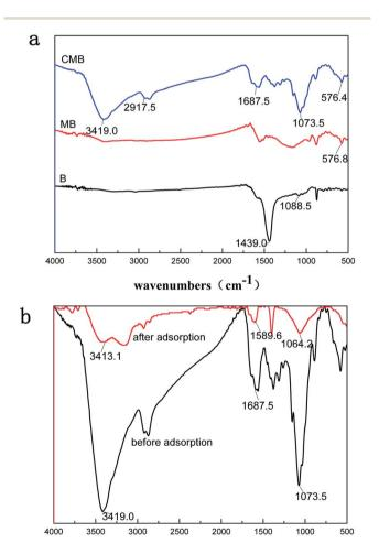
Fig. 3 (a) FTIR spectra of B, MB and CMB, (b) FTIR spectra of CMB before and after adsorption.
