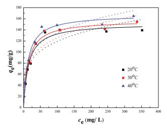
Fig. 9 Langmuir isotherm (solid line) and Freundlich isotherm (dash line) for the adsorption of Cr(vı) on CMB (reaction conditions:  $c_0=20-500$  mg L<sup>-1</sup>; V=50 mL; m=50 mg; t=6 h; pH = 2; T=20, 30, 40 °C).
