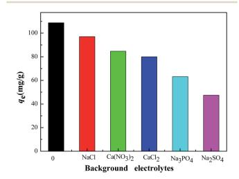
Fig. 11 Effect of background electrolyte (NaCl, Ca(NO<sub>3</sub>)<sub>2</sub>, CaCl<sub>2</sub>, Na<sub>3</sub>PO<sub>4</sub>, Na<sub>2</sub>SO<sub>4</sub>) on the Cr(v<sub>I</sub>) adsorption by CMB. (Reaction conditions: electrolyte concentration 0.01 mol L<sup>-1</sup>;  $Cr(v_1)$  concentration  $c_0 =$ 150 mg L<sup>-1</sup>; V = 50 mL; m = 50 mg; T = 30 °C; pH = 2).
