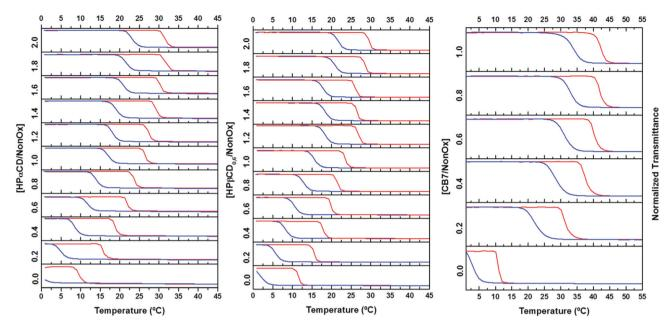
Fig. 5 Turbidimetry studies of 5 mg  $mL^{-1}$  solutions of PEtOx<sub>90</sub>-ran-PNonOx<sub>12</sub> with increasing cavitand/NonOx molar ratios. The heating and cooling ramps are represented by the top (red) and bottom (blue) curves, respectively. Rate: 1 K min<sup>-1</sup>,  $\lambda$  = 700 nm. At least 1.2 equivalents of HP $\alpha$ CD or  $HP\beta CD$  are necessary to keep the solution transparent at room temperature, in contrast to less than 0.2 equivalents of CB7.
