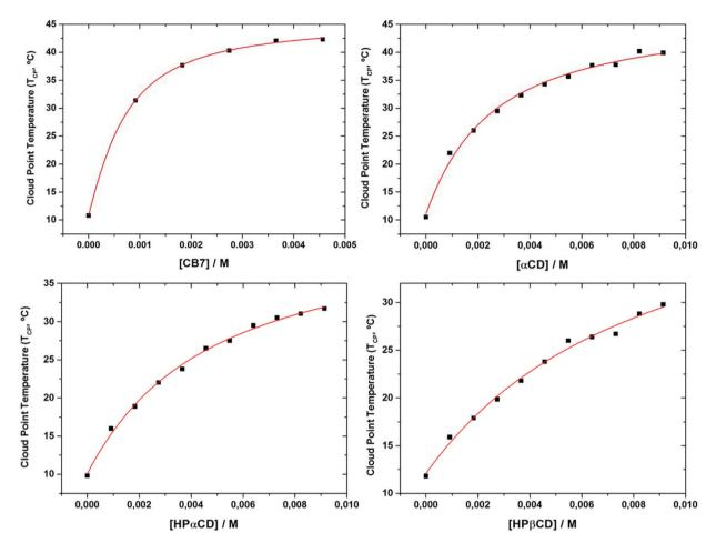
Fig. 7 Turbidimetry titration curves corresponding to 5 mg mL<sup>-1</sup> solutions of PEtOx<sub>90</sub>-ran-PNonOx<sub>12</sub>, and non-linear curve fitting based on egn (6). The average stability constants between the copolymer nonyl chains and cavitands follow the order: CB7  $\gg \alpha$ CD > HP $\alpha$ CD > HP $\beta$ CD.
