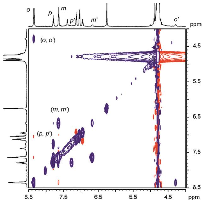
Fig. 5 Selected region of ROESY  $^1\text{H}$  NMR spectrum of complex  $\mathbf{11} \subset \alpha, \alpha, \alpha, \alpha\text{-}2$  in the presence of free  $\mathbf{11}$  in excess. The cross-peaks resulting from chemical exchange between protons of free and included  $\mathbf{11}$  are indicated. Primed letters correspond to signals of the protons in the complex.
