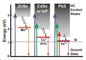
Fig. 8 Possibilities for semiconductor-dopant combinations indicating potential for covering more of the solar spectrum with for instance InP doped with Cu<sup>+</sup>. Reproduced with permission from ref. 196.
