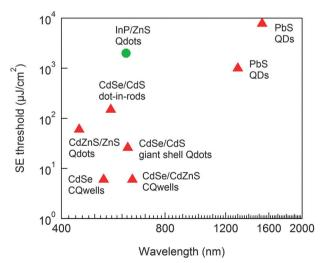
Fig. 11 Stimulated emission thresholds as a function of wavelength for InP/ZnS QDs,  $^{213}$  PbS QDs (1.3  $\mu m$ , ref. 227 and 1.52  $\mu m$ , ref. 218), CdSe/CdS dot-in-rods, 217 CdZnSe/ZnS QDs, 31 giant shell CdSe/CdS QDs, 228 CdSe/ CdZnS CQwells,<sup>225</sup> and CdSe CQwells,<sup>28</sup> highlighting both the lack of heavy-metal-free and the high threshold and scarce reports of NIR NC gain media
