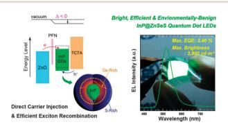
Fig. 5 Architecture of InP/ZnSeS QD-based LEDs with ZnO and 4.4',4''-tris(N-carbazolyl)triphenylamine (TCTA) as electron and hole transport layers, respectively, used to achieve an EQE of 3.46%. Reproduced with permission from ref. 158.
