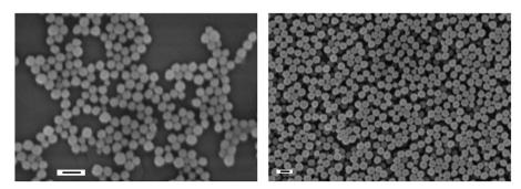
Fig. 3 Scanning electron micrographs of PMGVL latexes prepared with KPS (PDL, left) and AIBN (ADL, right); the bars indicate 200 nm.
