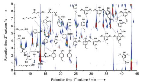
Fig. 7 Speciation of the products obtained from the catalytic biorefining of poplar wood in the presence of RANEY® Ni at 180 °C for 3 h (2-PrOH/H<sub>2</sub>O, 7:3, v/v). Reproduced with permission from ref. 35. Copyright 2014, Wiley-VCH Verlag GmbH & Co. KGaA, Weinheim.
