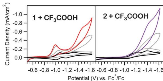
**Fig. 3** Acid titrations of 0.5, 4, and 10 eq. of [CF<sub>3</sub>COOH] into equimolar solutions of **1** and **2** (0.39 mM). The black traces are the respective acid-free voltammograms. Voltammograms recorded at 100 mV s<sup>-1</sup> in 100 mM [Bu<sub>4</sub>N][PF<sub>6</sub>] CH<sub>3</sub>CN solutions.
