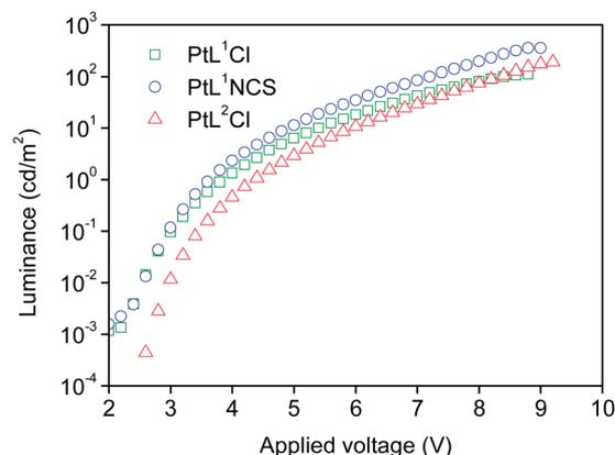
Fig. 7 Luminance versus applied voltage of the OLEDs using the neat complexes as emitting layers. The device incorporating **PtL<sup>1</sup>Cl** is shown in green, **PtL<sup>1</sup>NCS** is in blue, and **PtL<sup>2</sup>Cl** in red.
