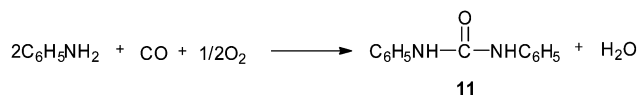
Scheme 5 Reagents and conditions: aniline (53.8 mmol), catalyst 5% Pd/C ( 5.0 \times 10^{-3} \text{ g cm}^{-3} ), NaI (0.87 mmol), DMF ( 95 \text{ cm}^3 ), \text{CO} : \text{O}_2 pressure (41 bar) ( \text{CO} : \text{O}_2 , 5 : 1), temp. 100^\circ\text{C} , time 2 h.
