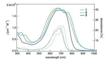
Fig. 2 UV-vis-NIR absorption spectra of 1-3 in  $CH_2Cl_2$  (dashed lines) and absorption spectra of thin-film samples on a quartz substrate (solid lines).
