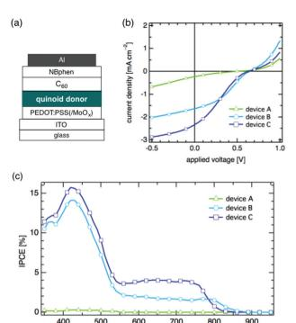
Fig. 3 The configuration of the fabricated OSC devices A, B, and C using the quinoid materials 1, 2, and 3, respectively, as a donor layer (a), J-V characteristics (b) and IPCE profiles (c) of the devices. For devices B and C, a molybdenum oxide (MoO<sub>x</sub>) layer was inserted between the PEDOT:PSS and the quinoid donor layers.
