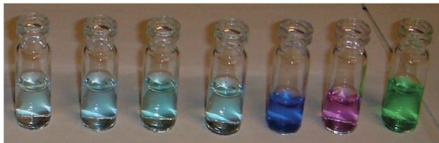
Fig. 15 Colour change of [\text{Cu}(\mathbf{94})](\text{BF}_4)_2 \cdot \text{MeCN} ( 10^{-3} M) upon the addition of different anions in MeCN. From left to right: free receptor; +1 eq. \text{F}^- ; +1 eq. \text{Cl}^- ; +1 eq. \text{Br}^- ; +1 eq. \text{CN}^- ; +2 eq. \text{CN}^- ; +1 eq. \text{I}^- . Reproduced with permission from Chem. Commun. 2011, 47 , 3805–3807. © Royal Society of Chemistry.
