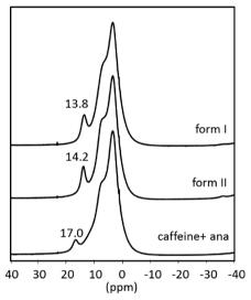
Fig. 3 <sup>1</sup>H magic angle spinning (MAS) NMR spectra of the cf:ana cocrystal form I (above) and form II (middle) and the superimposed spectra of the reactants (below) without the spinning sidebands.
