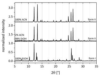
Fig. 7 PXRD patterns of cf:ana form II with different solvents (250  $\mu$ L) added to 1 g of the reactant mixture: acetonitrile (ACN), ethanol and acetonitrile (49:1, corresponding to the volumes of the solvents), and ethanol.
