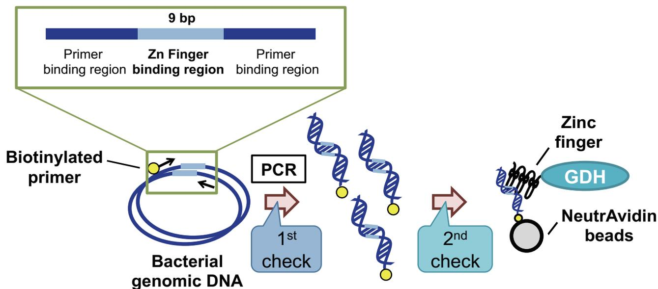
Fig. 1 Schematic of our detection system. The system that we designed in this study involved two steps: 1. PCR amplification of a target genomic region of pathogenic bacteria that included a ZF recognition sequence and 2. electrochemical detection of the PCR products using ZF-GDH.
