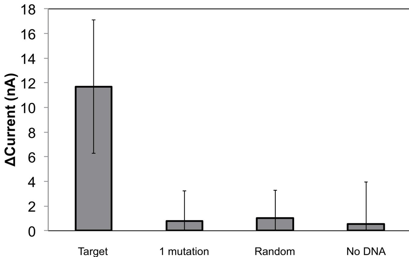
Fig. 3 Sequence specificity of Zif268-GDH with our electrochemical assay. A total of  $10^{10}$  copies of synthetic oligonucleotides were analyzed. Error bars indicate standard deviations ( $n = 3$ ).
