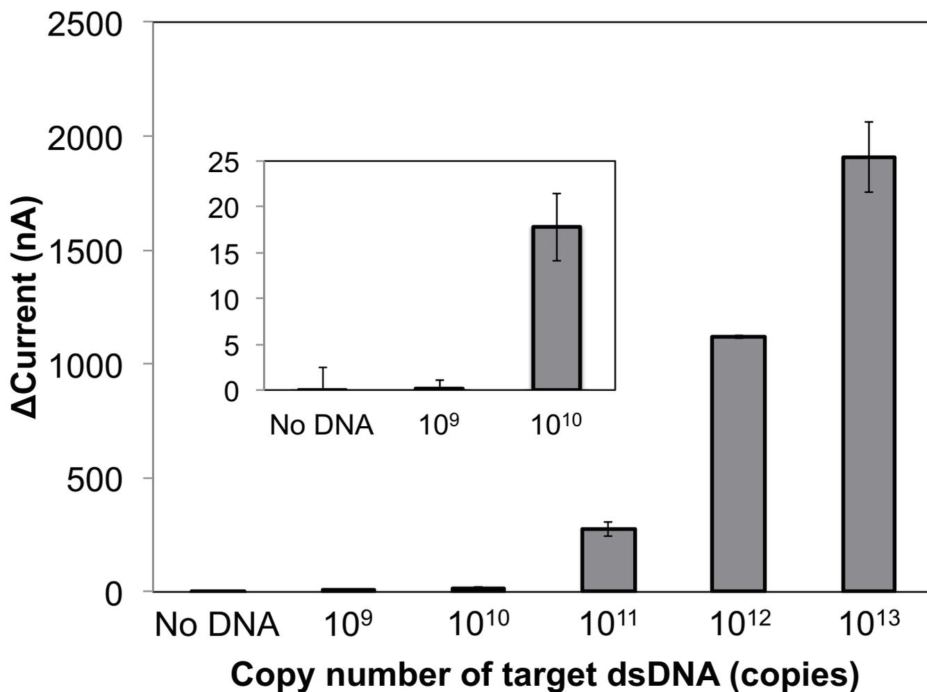
Fig. 2 Electrochemical detection of synthetic oligonucleotides that included the Zif268 recognition region. Delta current is the difference in current between before adding glucose and the plateau signal after adding 100 mM glucose. Error bars indicate standard deviations (n = 3).
