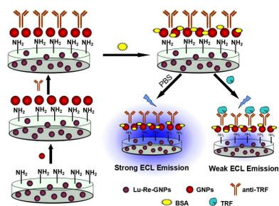
A disposable label-free electrochemiluminescent immunosensor based on luminol-reduced gold nanoparticles was designed for human transferrin detection.
