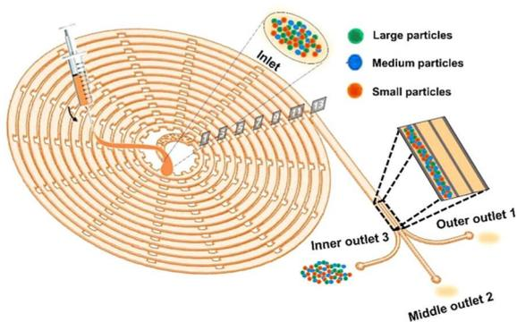
Fig. 6 A scheme of the spiral channel for high-throughput cell manipulation.<sup>31</sup> Reprinted and adapted with permission from ref. 31. Copyright 2024 American Chemical Society.
