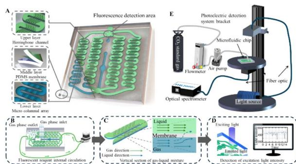
Fig. 2 High-precision, dynamic CO<sub>2</sub> sensing via cyclic microfluidic fluorescence: (A) a cyclic chip, (B) flow directions, (C) phase mixing, (D) intensity detection and (E) a full system platform.<sup>17</sup> Reprinted and adapted with permission from ref. 17. Copyright 2024 Elsevier B.V.
