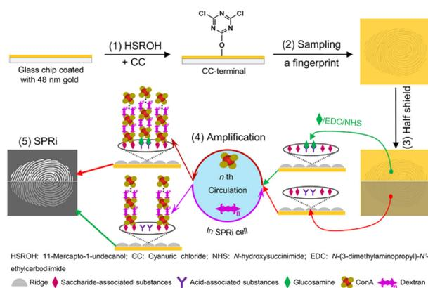
Fig. 9 Schematic of the chemical imaging of fingerprints with SPRi combined with a CS<sup>3</sup>A strategy.<sup>68</sup> Reprinted and adapted with permission from ref. 68. Copyright 2022 American Chemical Society.
