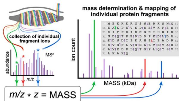
Fig. 12 A schematic of Orbitrap-based mass spectrometry analysis of the fragment ions of phosphoglycerate mutase.<sup>76</sup> Reprinted and adapted with permission from ref. 76. Copyright 2020 American Chemical Society.
