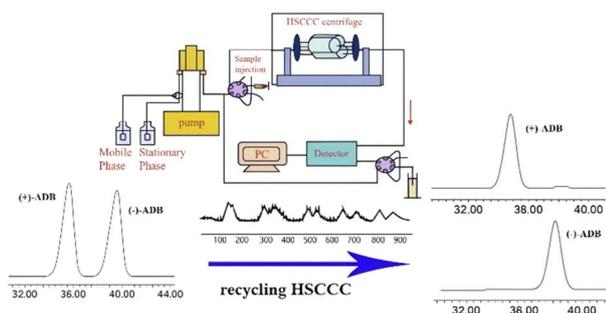
Fig. 7 Schematic of the recycling HSCCC for ADB enantiomer separation.<sup>53</sup> Reprinted and adapted with permission from ref. 53. Copyright 2015 Elsevier B.V.
