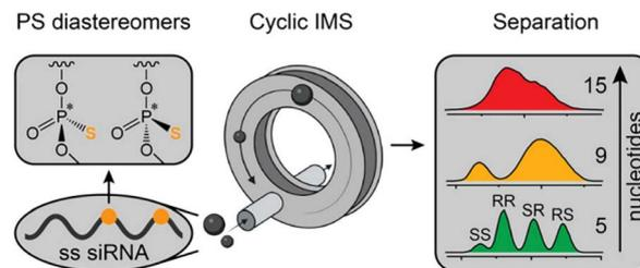
Fig. 8 Schematic of cIMS for phosphorothioate diastereomer separation in siRNA.<sup>58</sup> Reprinted and adapted with permission from ref. 58. Copyright 2025 American Chemical Society.
