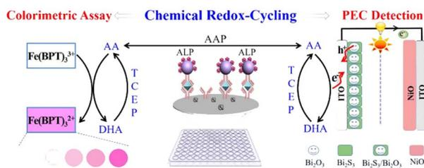
Fig. 5 Scheme of a chemical redox cycling biosensor integrated self-powered photoelectrochemical and colorimetric immunoassay.<sup>23</sup> Reprinted and adapted with permission from ref. 23. Copyright 2025 American Chemical Society.
