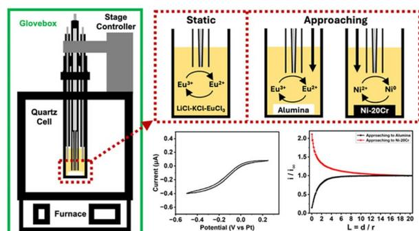
Fig. 11 A schematic of the CV method for monitoring of molten chloride salt chemistry and corrosion using a microelectrode.<sup>73</sup> Reprinted and adapted with permission from ref. 73. Copyright 2025 American Chemical Society.
