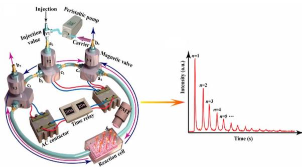
Fig. 4 Schematic of a gas-phase CCL system regulated by pump valves.<sup>21</sup> Reprinted and adapted with permission from ref. 21. Copyright 2014 American Chemical Society.
