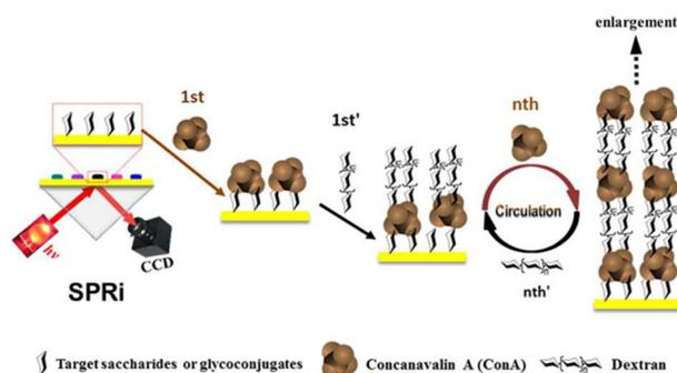
Fig. 3 Scheme of the signal stepwise amplification in surface plasmon resonance imaging detection of saccharides and glycoconjugates.<sup>20</sup> Reprinted and adapted with permission from ref. 20. Copyright 2016 American Chemical Society.
