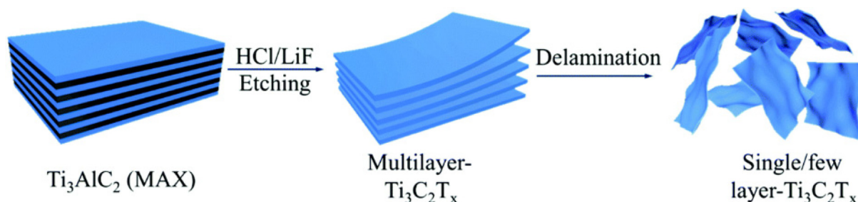
Fig. 5 Scheme of the fabrication procedure of MXenes. This figure has been reproduced from ref. 142 with permission from the Journal of Materials Chemistry C, copyright 2019.
