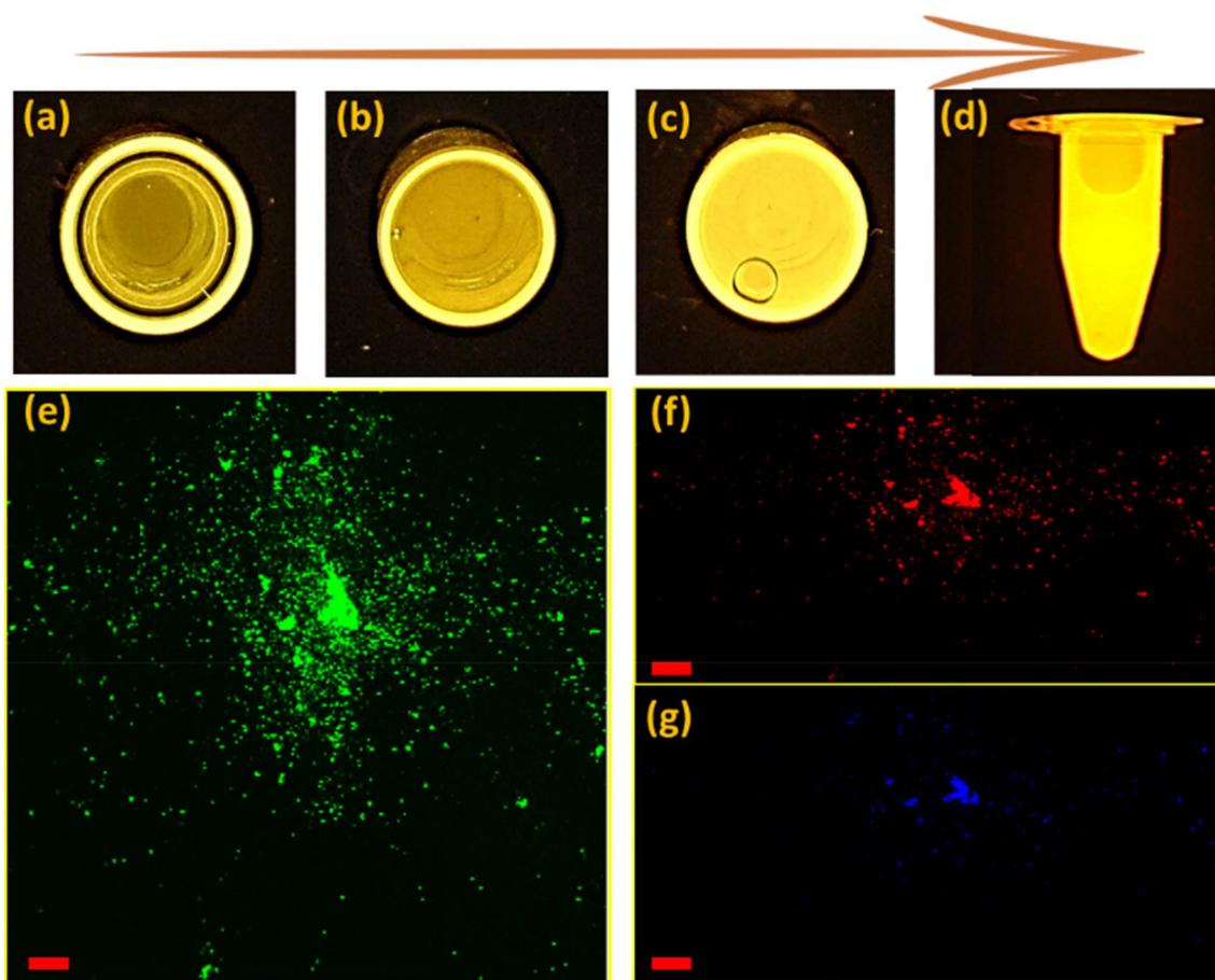
**Fig. 5** Luminescent and fluorescent images of rGO–TiO<sub>2</sub> (brookite). Increase in the luminescence of quantum GO–brookite particles is correlated to the enhancement in intensity of particle concentration from (a) to (d) resulting from the quantum confinement of GO and TiO<sub>2</sub> particles. The multi-emissive nature of the particles signifying photoswitchable energy states at the rGO–brookite interface.
