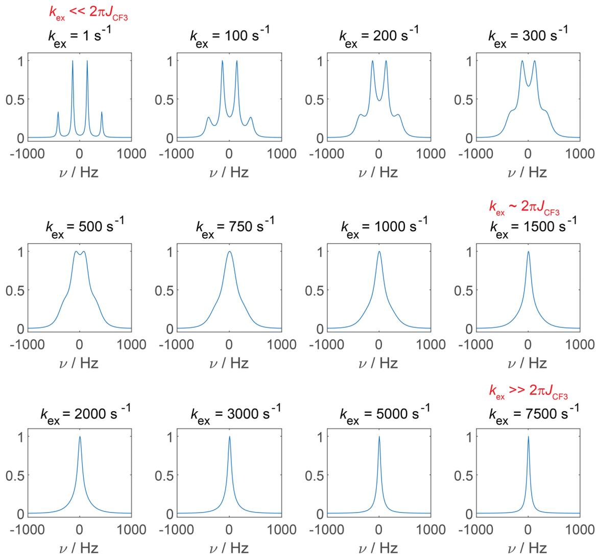
Fig. 2 Simulation of the  $^{13}\text{C}$  NMR spectrum of a  $\text{CF}_3$  group affected by  $^{19}\text{F}$  SD assuming a  $^{19}\text{F}$ – $^{13}\text{C}$  J-coupling constant of 280 Hz and a linewidth of 10 Hz ( $\text{FWHM} = 1/(\pi T_2)$ ). The spectra have been simulated as a function of the SD rate constant  $k_{\text{ex}}$ .
