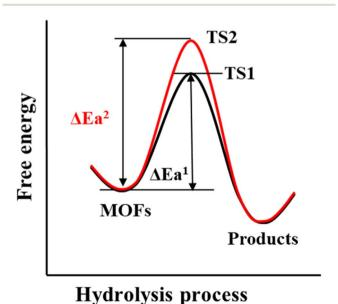
Scheme 3 The definition and optimization of the kinetic stability of MOFs to water. Black line represents the kinetic stability of a given MOF to water, which refers to the  $\Delta \text{Ea}^1$  (activation energy) of its hydrolysis reaction. The red line represents the optimized kinetic stability of the MOF through enhancing its activation energy ( $\Delta \text{Ea}^2 > \Delta \text{Ea}^1$ ).
