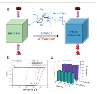
Fig. 41 (a) Coating HPMCP on SIFSIX-3-Ni. (b) The breakthrough curves of SIFSIX-3-Ni and HPMCP/SIFSIX-3 for  $CO_2/N_2$  (1:99) under different humid conditions. (c) The HPMCP/SIFSIX-3-Ni recyclability tests for humid 1%  $CO_2/99\%$   $N_2$  and 15%  $CO_2/85\%$   $N_2$  gas mixtures (regeneration at 80 °C). Reproduced from ref. 254 with permission from the American Chemical Society, Copyright 2020.
