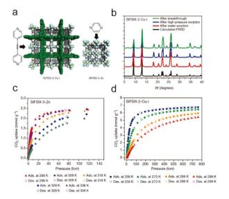
Fig. 33 (a) The structure of SIFSIX-2-Cu-i and SIFSIX-3-Zn. (b) PXRD patterns of SIFSIX-2-Cu-i after breakthrough experiments, high-pressure absorption, and water adsorption. (c) and (d) The  $\rm CO_2$  sorption isotherms of SIFSIX-3-Zn (c) and SIFSIX-2-Cu-i at different temperatures. Reproduced from ref. 213 and 214 with permission from Springer Nature, Copyright 2015.
