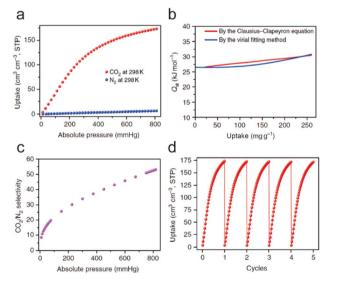
Fig. 34 (a) The  $\rm CO_2$  and  $\rm N_2$  adsorption isotherms for FJI-H14 at 298 K. (b) The isosteric heat of  $\rm CO_2$  adsorption ( $\rm Q_{st}$ ) for FJI-H14. (c) The IAST selectivity of FJI-H14 for  $\rm CO_2/N_2$  (15:85). (d) 5 Cycles of  $\rm CO_2$  adsorption for FJI-H14 at 298 K. Reproduced from ref. 136 with permission from Springer Nature, Copyright 2017.
