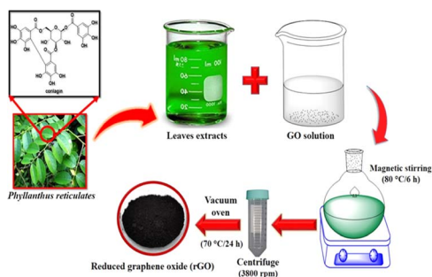
Fig. 6 Green reduction of graphene oxide (GO) using an aqueous leaves extract.
