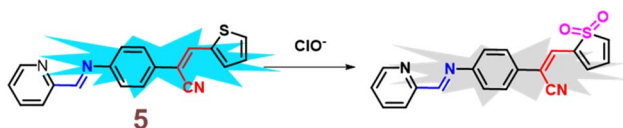
Fig. 8 Proposed sensing mechanism of 5 with \text{ClO}^- ions.
