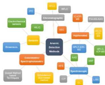
Fig. 3 Different methods of arsenic detection and determination.
