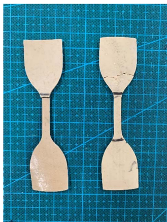
Fig. 33 Dumbbell test piece of (Left) natural rubber and (Right) natural rubber nano cellulose composite material. 180
