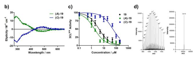
Fig. 4 Evaluation of the chiral enantiomers of compound 19. (a) Synthetic strategy for separation of the enantiomers. (b) Circular dichroism spectra of the enantiomers (A)-19 and (C)-19 in methanol. (c) Dose–response curves of 19, (A)-19, and (C)-19 against 3CL<sup>pro</sup>. (d) Original and deconvoluted mass spectrum of 3CL<sup>pro</sup> upon incubation with (A)-19.
