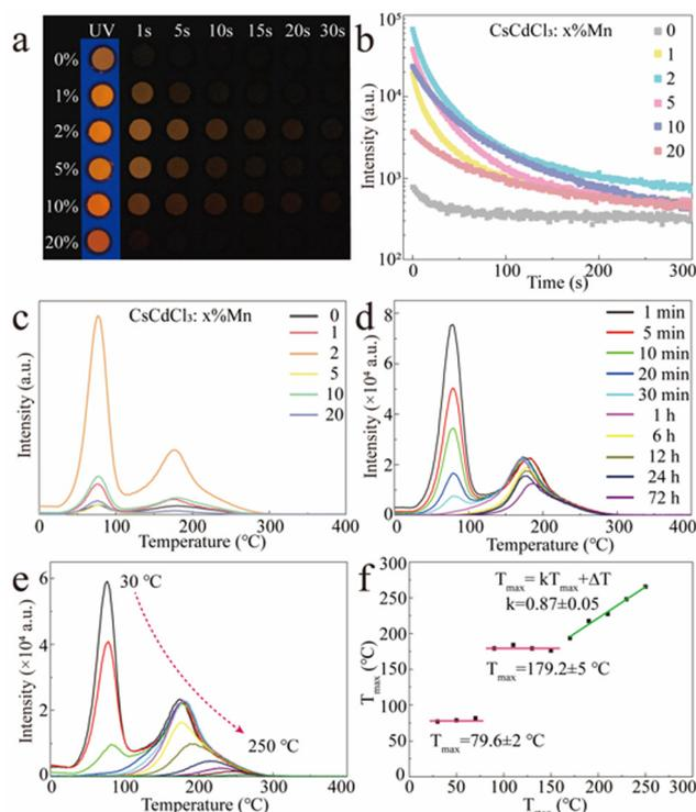
**Fig. 3** (a) Afterglow photographs of CCCP: $x\%$ Mn ( $x = 0-20$ ) crystals taken under UV excitation and at different times after the removal of the UV light. (b) Afterglow decay curves, and (c) TL curves of CCCP: $x\%$ Mn ( $x = 0-20$ ). (d) The TL curves of CCCP:2%Mn obtained at various delay times from 1 min to 24 h. (e) The TL curves of CCCP:2%Mn recorded with preheating at various temperatures. (f) The  $T_{\max} - T_{\text{stop}}$  plot of CCCP:2%Mn.
