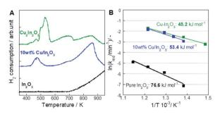
Fig. 5 Kinetics analysis of each oxide in the reduction step. (A) H<sub>2</sub>-TPR profiles for Cu-In<sub>2</sub>O<sub>3</sub> (derived from Cu<sub>2</sub>In<sub>2</sub>O<sub>5</sub>), 10 wt% Cu/In<sub>2</sub>O<sub>3</sub> and In<sub>2</sub>O<sub>3</sub>. (B) Arrhenius plots for the reduction of Cu-In<sub>2</sub>O<sub>3</sub> (derived from  $Cu_2In_2O_5$ ), 10 wt%  $Cu/In_2O_3$  and  $In_2O_3$ .
