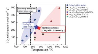
Fig. 2 Average CO<sub>2</sub> splitting rates on the Cu-In mixed oxide (this study) and on various oxides in earlier reports.
