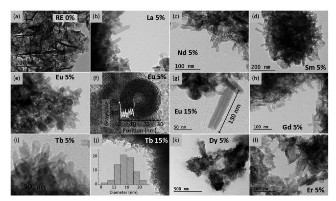
Fig. 2 Transmission electron micrographs comparing the morphology of (a) ZnAl-BTC and (b-l) ZnAlLn<sub>XX</sub>-BTC-P123 (Ln = La and from Nd to Er, X = 5 or 15%). The pixel profile along the diameter of a nanotube is shown on (f). The inset in (j) displays the external diameter distribution histogram of the ZnAlTb<sub>15X</sub>-BTC-P123 nanotubes.
