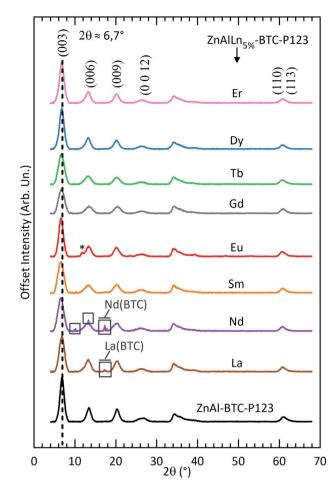
Fig. 1 Powder X-ray diffraction patterns of ZnAl-BTC-P123 and  $ZnAlLn_{5\%}-BTC-P123$  (Ln = La and from Nd to Er). The Bragg peaks inside the rectangles are attributed to the formation of the respective Ln(BTC) complex.35-37 The starred peak are ascribed to a carbonateintercalated LDH phase formed in the Eu<sup>3+</sup>-containing solid.
