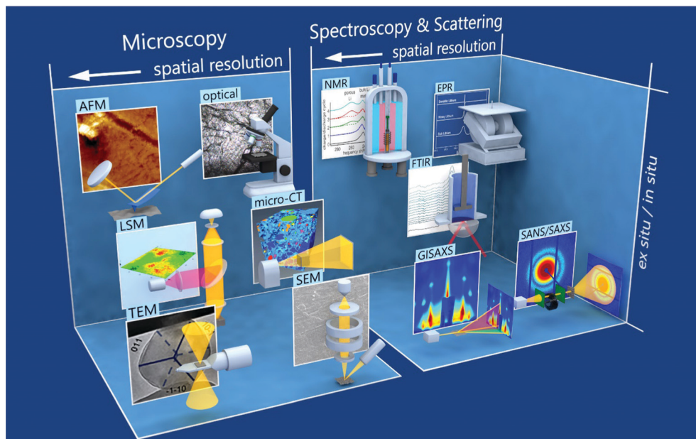
Fig. 1 Various methods for studying metallic lithium are schematically presented, along with a typical result, and are divided into microscopic and spectroscopic & scattering techniques. Microscopic techniques include transmission electron microscopy (TEM), 14,15 scanning electron microscopy (SEM), 9 laser scanning microscopy (LSM), 16 micro computed tomography (micro-CT), 17 atomic force microscopy (AFM), 18,19 and optical microscopy. 20 Spectroscopic & scattering techniques include grazing-incidence small angle X-ray scattering (GISAXS), 21 small-angle neutron scattering (SANS), 22 Fourier-transformed infrared (FTIR), 8,23 nuclear magnetic resonance (NMR), 24,25 and electron paramagnetic resonance (EPR). 24 Spectroscopy. Within the classifications and individual rows, the spatial resolution becomes higher the more left the method is depicted. From bottom to top, it is indicated if a technique is rather used ex situ or in situ . Details on the different characterization techniques are given in Section 5.
