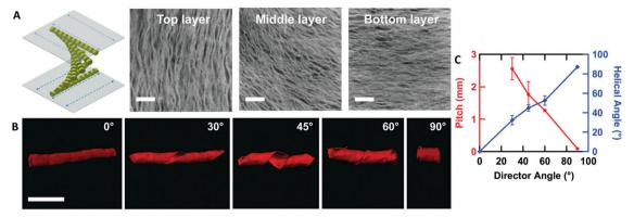
Fig. 4 Twisted aligned PAAm hydrogels. (A) Twisted aligned hydrogels induced by twisted oriented LCLCs (confocal images indicate the Z-stacking structure of hydrogels from top layer to bottom layer, scale bar 10 μm). (B) Confocal images of 2D hydrogel films forming 3D shapes by varying the cutting angle from 0° to 90° (scale bars 2 mm). (C) Pitch and helical angle of the 3D shapes measured as a function of cutting angle (the pitch of the 0° sample is infinite).
