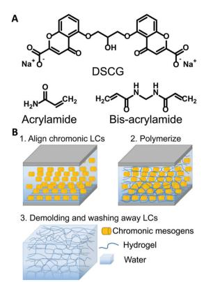
**Fig. 1** Schematic of the templating process. (A) Chemical structure of DSCG and monomers. (B) Illustration of the synthesis of anisotropic hydrogels templated by chromonic liquid crystals.
