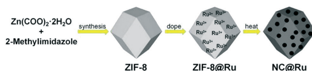
Fig. 1 Schematic diagram of preparation process.
