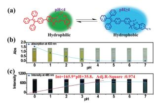
Fig. 2 (a) Illustration of switching between the ring-closed and protonated ring-open forms of TPE-Sp-CN at different pH values. (b) The plot of the absorption at 433 nm of the **TPE-Sp-CN** solutions (1 mL,  $1 \times 10^{-4}$  M) treated with 0.2 mL water samples with different pH values (0 to 7). (c) The plot of the emission intensity of **TPE-Sp-CN** in acid solutions ( $V_{MeCN}$ :  $V_{acid}$ water = 1:9) against pH (0 to 7).
