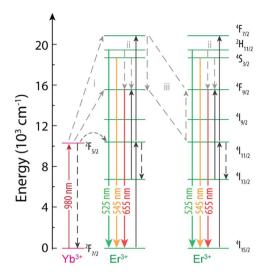
Fig. 5 Partial energy level diagram of Yb<sup>3+</sup> and Er<sup>3+</sup> in NaYF<sub>4</sub>:Yb<sup>3+</sup>/Er<sup>3+</sup> NPs.<sup>68</sup> The mechanisms proposed in the literature as being responsible for the variation of the R/G ratio are shown.
