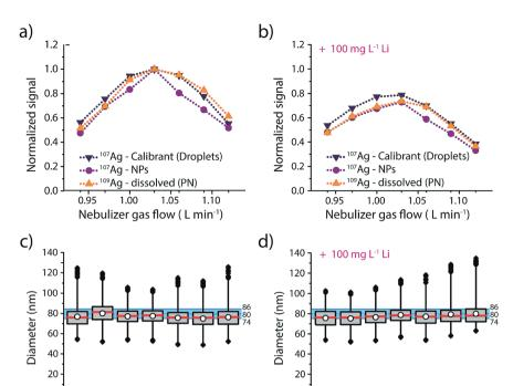
Fig. 3 (a) Normalised signal intensities recorded for Ag analyte in the form of NPs, microdroplets and enriched  $^{109}$ Ag solution without any additional matrix at nebulizer gas flow rates between 0.94 and 1.12 L min $^{-1}$ . (b) Same experiment as in (a), but with 100 mg L $^{-1}$  Li matrix. (c) and (d) Corresponding sizing of the 80 nm Ag NPs at different nebulizer gas flow rates. In both (c) and (d), the shaded blue area shows the expected NP diameter from the manufacturer.
