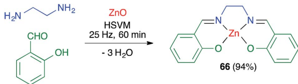
Scheme 46 Mechanochemical synthesis of a zinc-salen complex.
