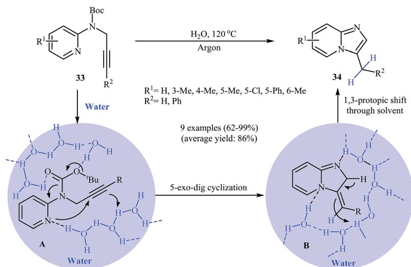
Scheme 12 Intramolecular hydroamination of Boc-protected *N*-propargylaminopyridines **33** in water.
