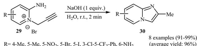
Scheme 10 Metal-free and aqueous synthesis of imidazo[1,2-*a*]pyridine **30** from *N*-propargylpyridiniums **29**.
