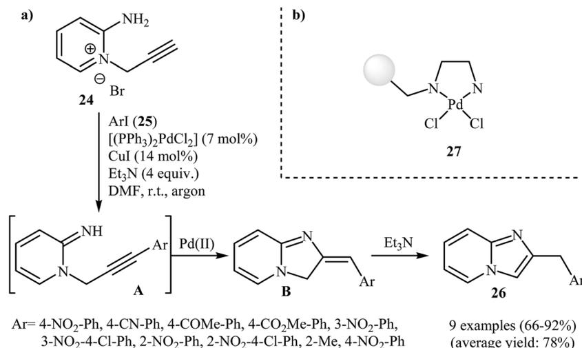
**Scheme 8** (a) Synthesis of 2-benzylimidazo[1,2-*a*]pyridines **26** through a tandem Sonogashira coupling/intramolecular cyclization/aromatization sequential process. (b) Chemical structure of polystyrene-supported palladium(II) ethylenediamine complex **27**.
