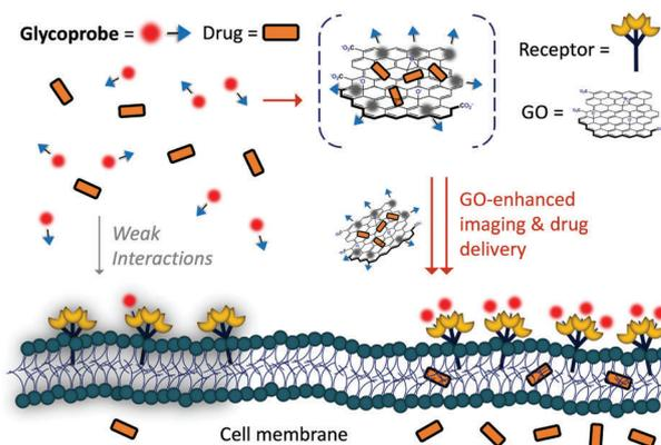
**Fig. 12** Schematic illustration of glycoprobe–GO composite material for targeted theranostics (combined imaging and drug delivery). Reproduced with permission from ref. 72 (*J. Mater. Chem. B*, 2015, **3**, 9182). Copyright: The Royal Society of Chemistry.
