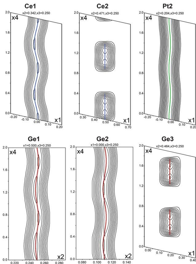
**Fig. 2** Sections of the Fourier maps (based on  $F_{\text{obs}}$ ) of the orthorhombic (3 + 1)D refinement with superspace group  $Cmc m(\alpha, 0, 0)0s0$  ( $\alpha = 1/2 a^*$ ) of the commensurately modulated structure of  $Ce_3Pt_4Ge_6$ . Summation over 100 pm of the projected directions was conducted. Contour lines for all atoms correspond to a difference of  $10 e \text{ \AA}^{-3}$ , each.
