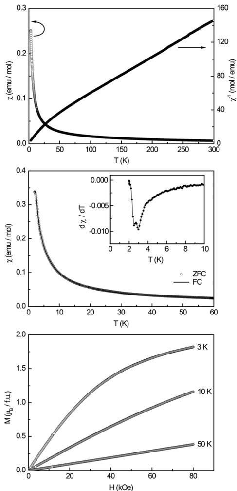
**Fig. 6** Magnetic properties of  $\text{Ce}_3\text{Pt}_4\text{Ge}_6$ : (top) Temperature dependence of the magnetic susceptibility  $\chi$  and its reciprocal  $\chi^{-1}$  measured with a magnetic field strength of 10 kOe; (middle) magnetic susceptibility in zero-field (ZFC) and field-cooled (FC) mode at 100 Oe; (bottom) magnetization isotherms at 3, 10, and 50 K.
