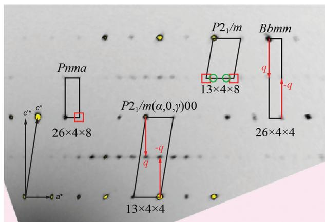
**Fig. 1** Sections of the (reconstructed) diffraction pattern of  $Ce_3Pt_4Ge_6$ . The different unit cells found in the literature are drawn to show the possible (mis)interpretations of the data. Also the monoclinic interpretation in superspace group  $P2_1/m(\alpha, 0, \gamma)00$  with  $\alpha = 1/4 a^*$  and  $\gamma = 1/2 c^*$  is shown.
