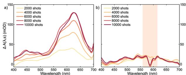
Fig. 3 Change in the absorption spectra of SNO thin crystals measured 28 ms after excitation for different number of 266 nm laser shots ( $1.4 \text{ mJ cm}^{-2}$ ) a) without using the NOPA photoreversion pulse and b) with the photoreversion pulse ( $2.8 \text{ mJ cm}^{-2}$ ). The spectral region covered by the NOPA is shaded. In this region, the scattered light coming from the NOPA beam reaching the detector produced fluctuations increasing the noise significantly.
