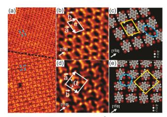
Fig. 1 (a) Overview STM image ( $30 \times 14 \text{ nm}^2$ ) for 1 ML Br<sub>4</sub>Py on Au(111), showing the co-existence of two different molecular arrangements, labelled phase I (top) and phase II (bottom). (b, c) and (d, e) Close-up STM images ( $5 \times 5 \text{ nm}^2$ ) and corresponding proposed molecular models for phase I and II, respectively. The STM images were taken at room temperature with U = -1.2 V, I = 60 pA.
