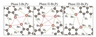
Fig. 3 DFT optimized intermolecular interactions for phase I and II formed by Br<sub>4</sub>Py and for phase III formed by Br<sub>2</sub>Py molecules. The intermolecular Br-Br and Br-H bonds are marked by red and green dashed lines, respectively
