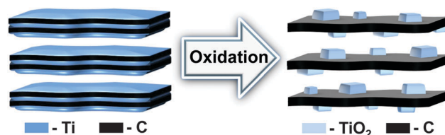
Fig. 1 Schematic of MXene oxidation and formation of oxide-graphitic disordered carbon hybrid structure.
