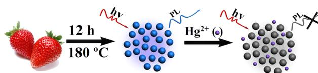
**Scheme 1** Schematic illustration of the preparation process for the FNCPs and their application for Hg<sup>2+</sup> detection.
