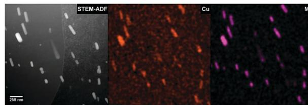
**Fig. 2** STEM-ADF image and the corresponding EDX elemental maps of a FIB specimen of AA 2024-T3 reveal plate-like precipitates in the aluminium matrix enriched with Cu and Mn. These plate type precipitates have been identified as the Al<sub>20</sub>Mn<sub>3</sub>Cu<sub>2</sub> type, which exhibit *cathodic* behaviour with respect to the matrix.
