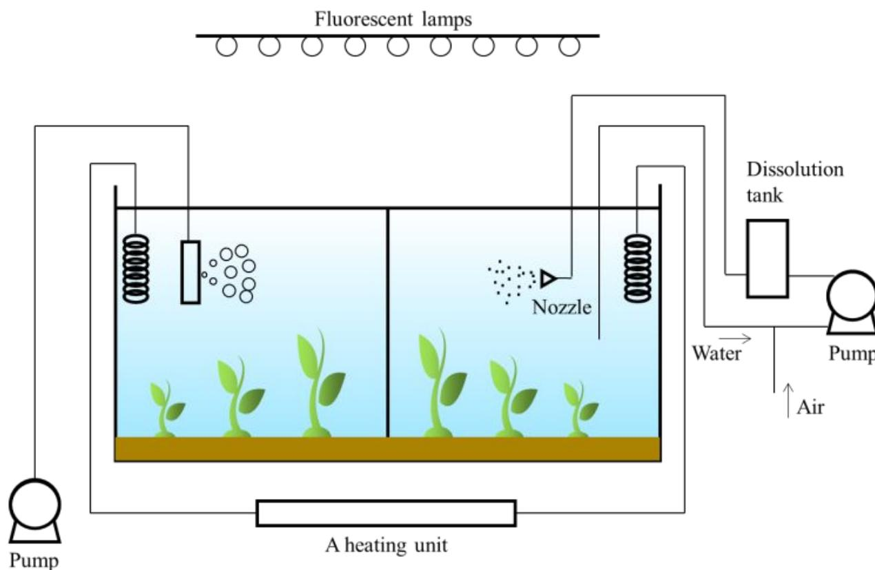
**Fig. 1** - The experimental setup for cultivation of submerged plants using two aeration systems (micro-nano bubble, right; macrobubble, left).
