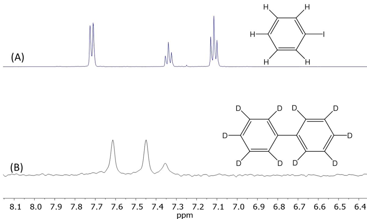
**Figure 5.** (A)  $^1\text{H}$  and (B) D NMR spectra of benzene- $d_6$  coupling to give exclusively biphenyl- $d_{10}$  in  $\text{CD}_2\text{Cl}_2$  (A) and  $\text{CH}_2\text{Cl}_2$  (B): reaction conditions:  $[\text{Pt catalyst}] = 0.010 \text{ M}$ ,  $[\text{PhI}(\text{OAc})_2] = 0.18 \text{ M}$  in  $1.0 \text{ mL C}_6\text{D}_6$  at  $100^\circ\text{C}$  after 24 h.
