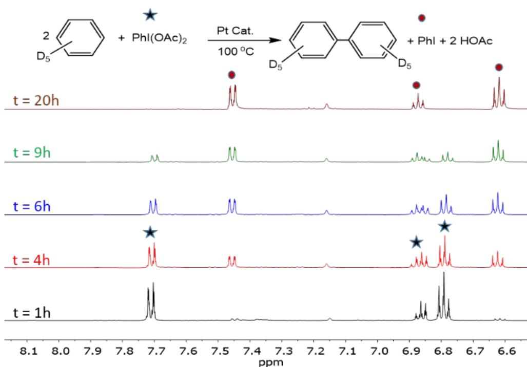
**Figure 1.**  $^1\text{H}$  NMR spectra of the reaction of  $\text{PhI}(\text{OAc})_2$  and  $[\text{PtMe}(\text{bhq})(\text{SMe}_2)]$ , **1** in  $\text{C}_6\text{D}_6$  at 100 °C; condition:  $[\mathbf{1}] = 0.010 \text{ M}$ ,  $[\text{PhI}(\text{OAc})_2] = 0.15 \text{ M}$  in  $\text{C}_6\text{D}_6$  (1.0 mL). Only aromatic region is shown.
