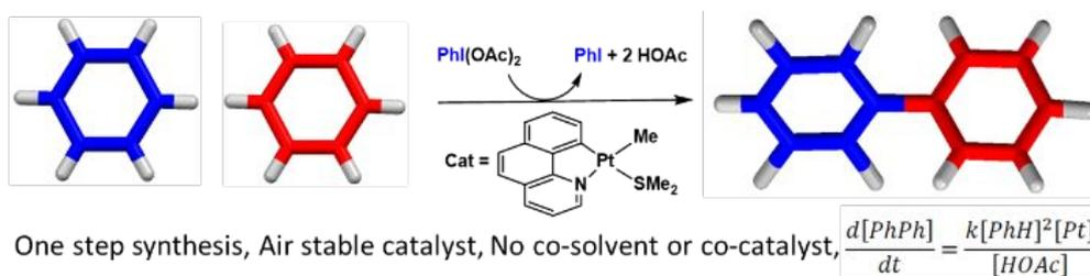
Pt-catalyzed direct coupling of benzene to biphenyl using  $\text{PhI}(\text{OAc})_2$  as oxidant in the absence of any acid as co-solvent or co-catalyst was mechanistically investigated showing first-order in Pt catalyst and second-order in benzene, which implicates the second C-H activation step as rate-limiting.
