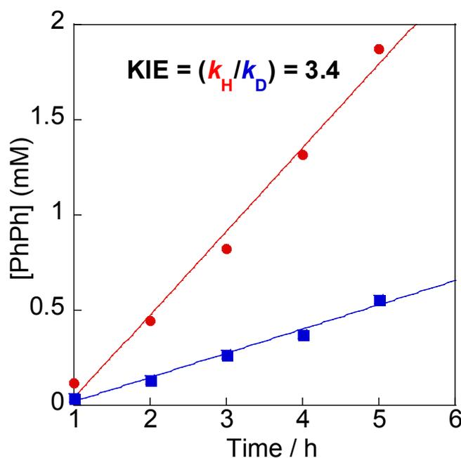
**Figure 3.** Kinetic isotope effect derived from initial rate measurements for coupling of benzene to form biphenyl using  $\text{PhI}(\text{OAc})_2$  as oxidant and Pt complex **1** as catalyst;  $[\text{benzene}] = 5.6 \text{ M}$ ,  $[\mathbf{1}] = 12.6 \text{ mM}$ ,  $[\text{PhI}(\text{OAc})_2] = 200 \text{ mM}$ .
