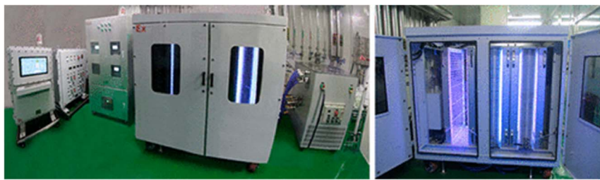
Fig. 15 Pictures of the production-scale photochemical skid. Reproduced from ref. 249 with permission from American Chemical Society.
