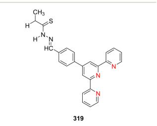
Fig. 22 Receptor 2-(4-(TPY)-4'-yl-phenyl)-*N*-methyl-3-thiosemicarbazone for detection of inorganic cation and fluoride anions.
