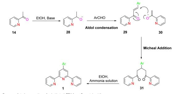
Scheme 9 Base-mediated preparation of substituted-TPY from 2-acetylpyridine.
