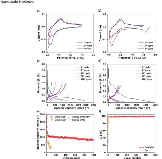
Fig. 4 Cyclic voltammetry diagrams of (a) Ge electrode and (b) Ge/CNT-1 electrode. Discharge—charge profiles of (c) Ge electrode and (d) Ge/CNT-1 electrode. (e) Cyclability with (f) coulombic efficiency of Ge electrode and Ge/CNT-1 electrode at C/5.
