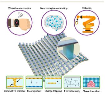
Fig. 1 Applications and mechanisms of flexible memristors.
